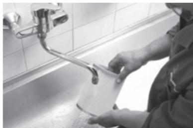
**Phase 6:** Check that filters are always clean, in order to avoid motor overheating. If the filters are dirty, you have to clean it immediately.
